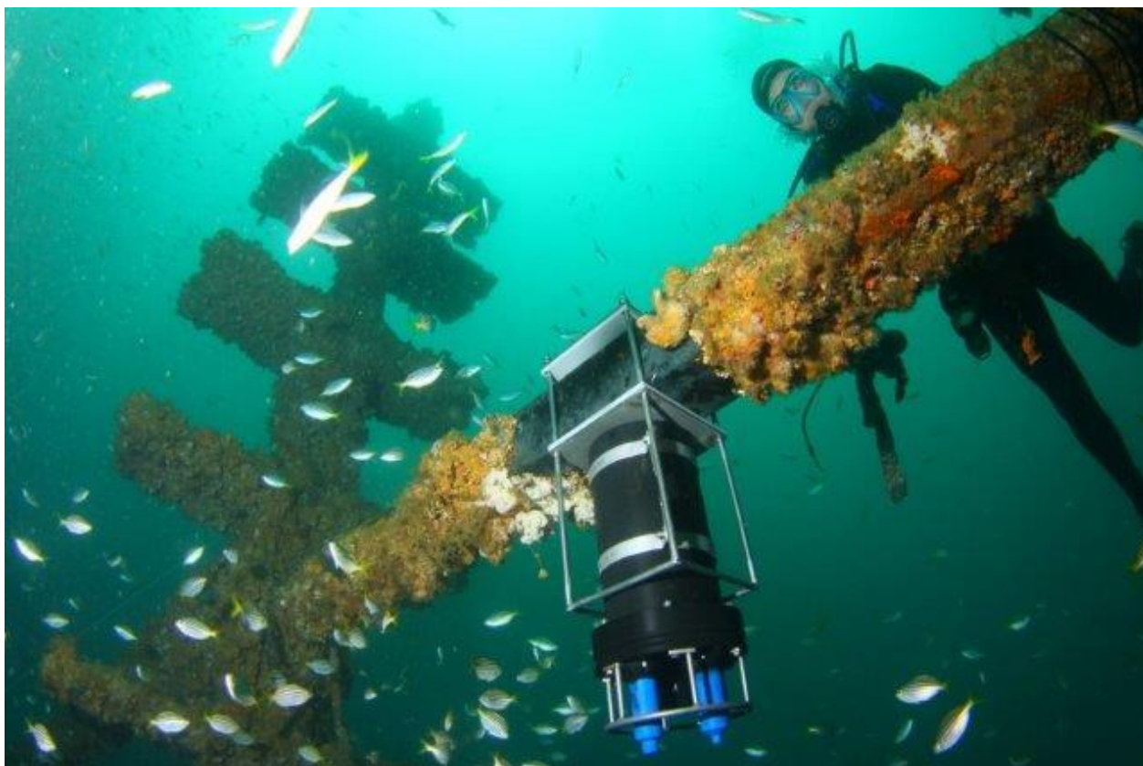
Figure 20. Vemco VR4 with a 10 year battery life and remote download capabilities fitted to the Sydney offshore artificial reef
