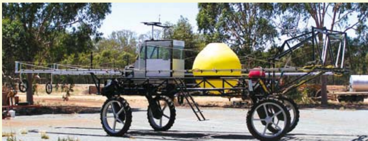
Wass's self propelled spray rig.
