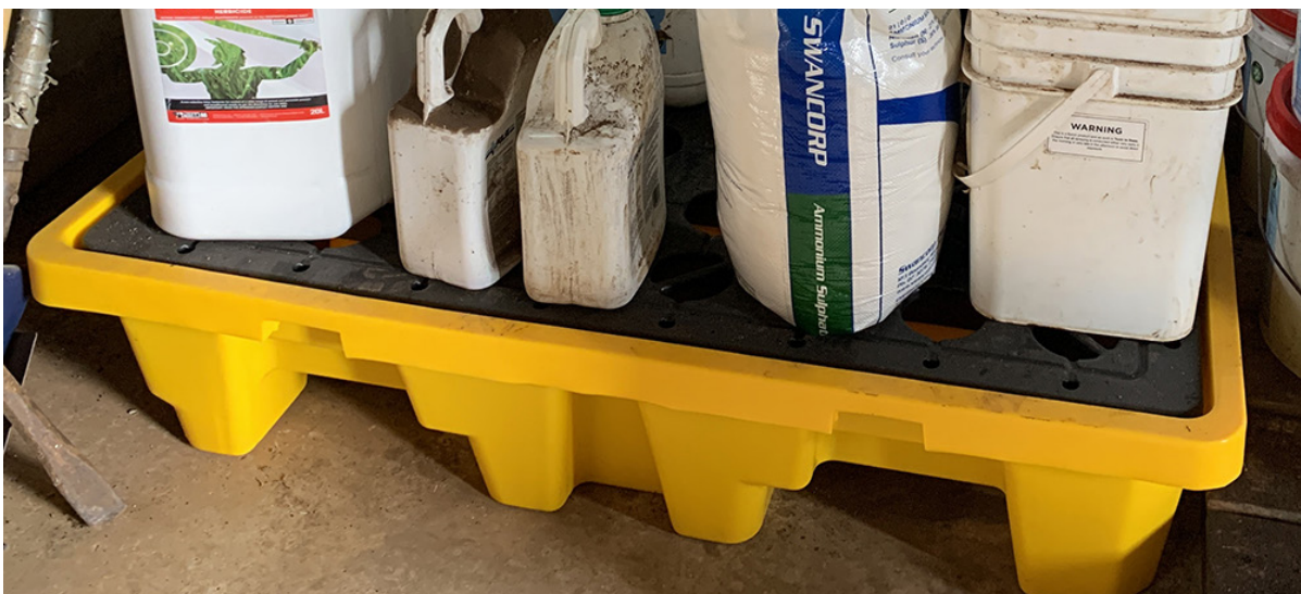
Figure 7. Bunded pallets underneath individual smaller containers, drums or barrels to capture leaks or spills.
