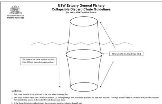
4. Not less than 400 mm of the chute must be submerged in the water when releasing fish. If the depth of the water to which fish are being released is less than 400 mm the chute must be submerged deep enough to ensure that fish are released below the water's surface.
